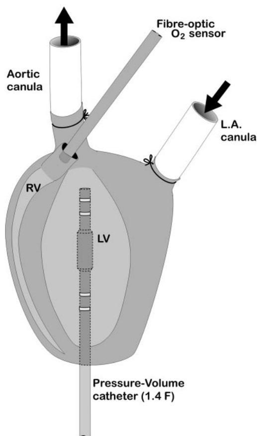
**FIG. 1.** Schematic of the isolated working mouse heart, showing the position of the pressure-volume catheter and oxygen probe in the left ventricle and pulmonary trunk, respectively. L.A., left atrial; LV, left ventricle; RV, right ventricle.
