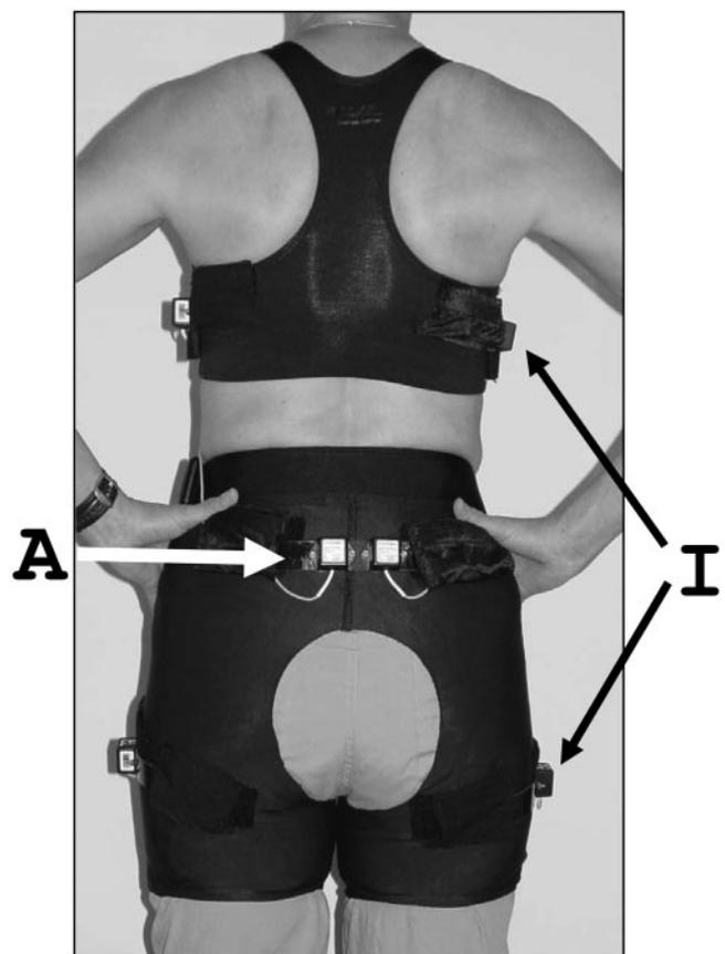
FIG. 1. Harnesses and sensor placement. Harnesses for accelerometers (A) and inclinometers (I). The harnesses are worn as “underwear.”
