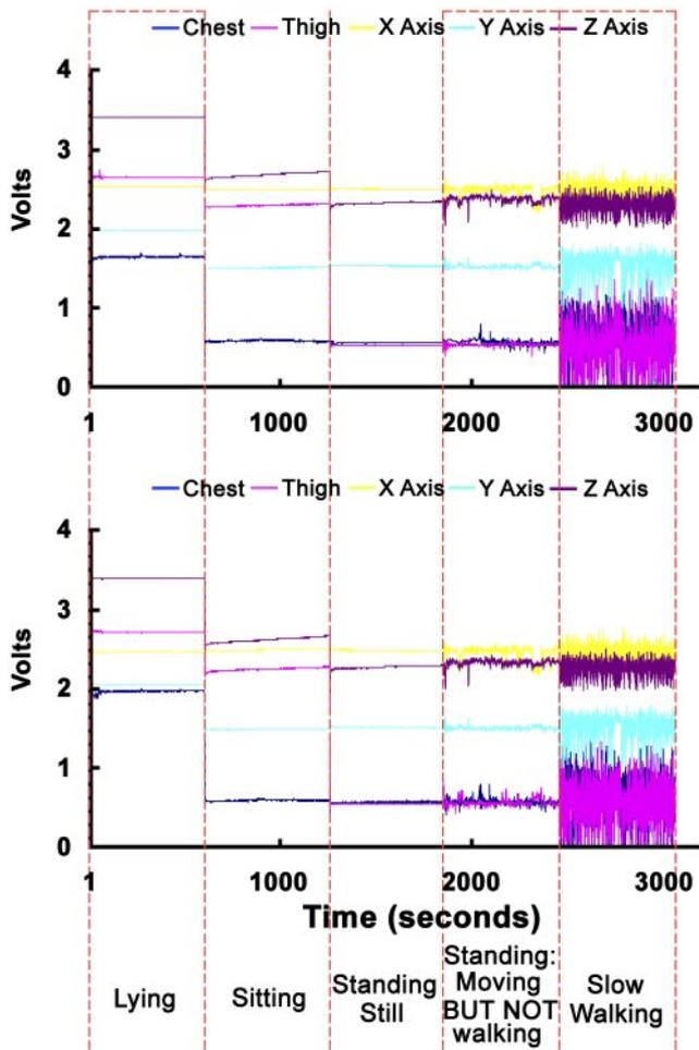
FIG. 2. Raw data stream from six sensors for different body postures and movements. A raw data stream from a subject lying still, sitting, standing still, standing while moving (but not walking), and walking. The top panel is from the left side of the body and the bottom panel from the right side of the body. (Please see <http://dx.doi.org/db07-0815> for a high-quality digital representation of this figure.)
